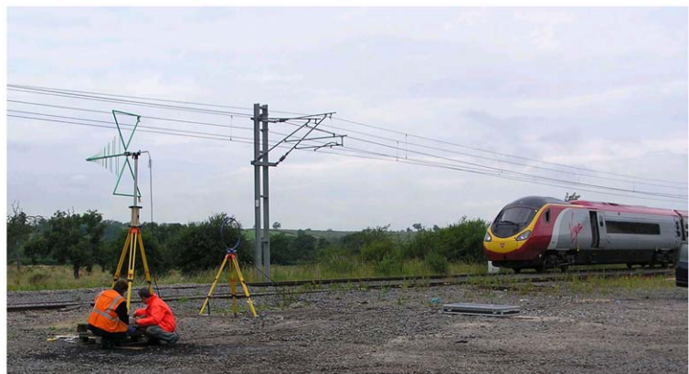
Figure 1: Radio Frequency emission measurements of a Class 390 Pendolino to EN50121:3-1:2000
