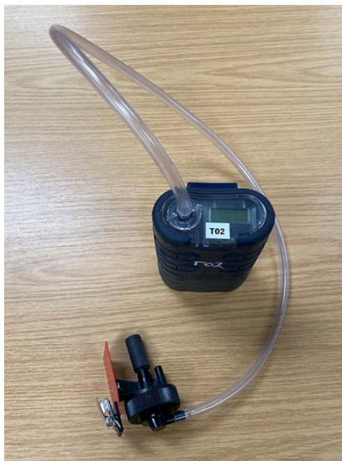
Figure 25 – Typical personal sample pump
