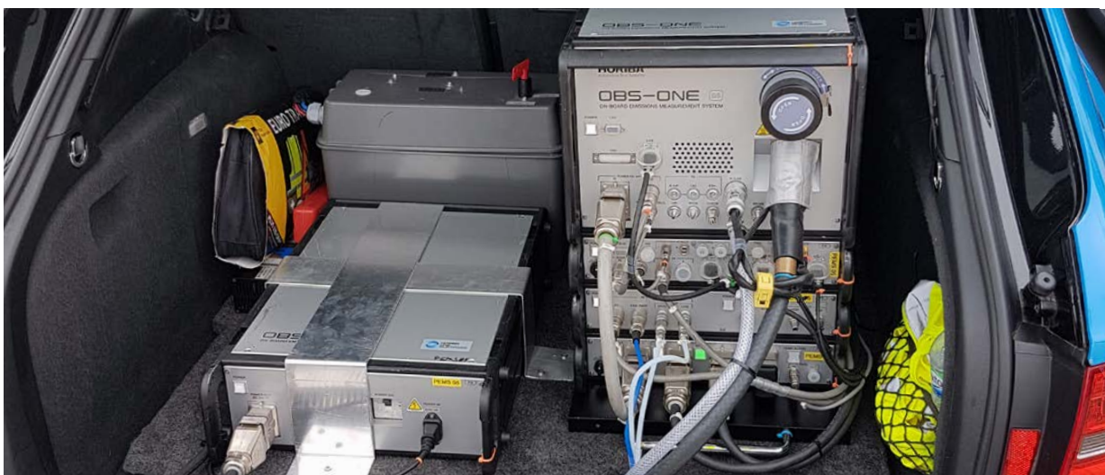
Figure 21 – Example of automotive PEMS equipment
