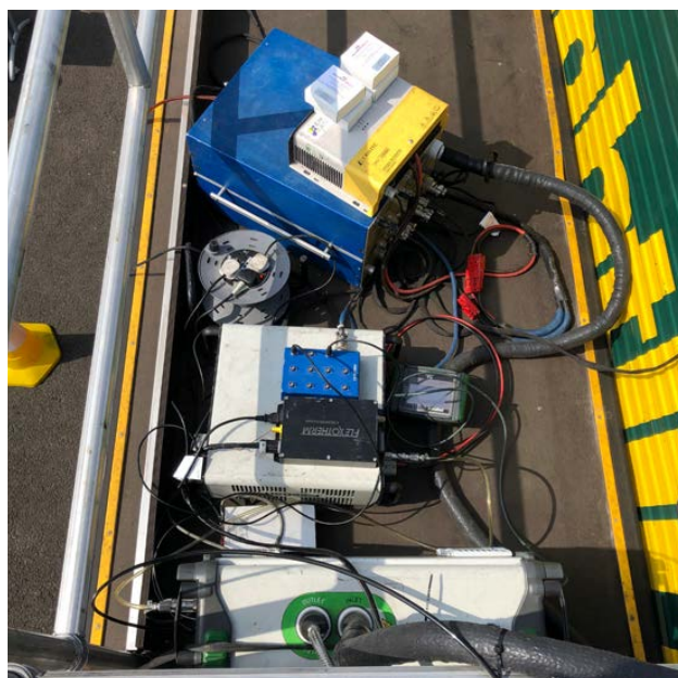
Figure 22 – PEMS setup on Class 66
