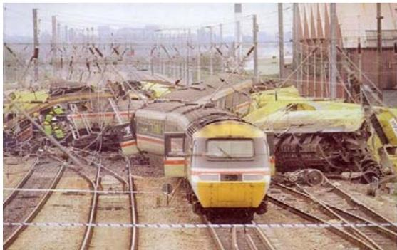
**Fig 1:** The train crash at Southall on 19 September 1997, where seven people lost their lives and many more were injured. This was due to non-compliance with rules such that the driver of an HST passed two red signals and collided with a freight train
